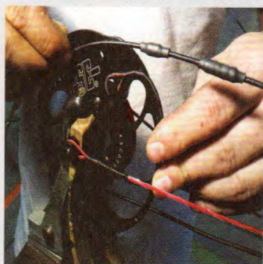
Step #24 Hook string on top cam string post.
