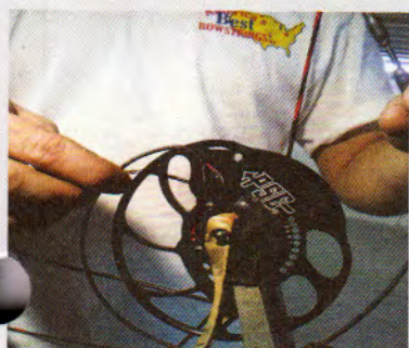
Step #25 Hook string on bottom cam string post.
