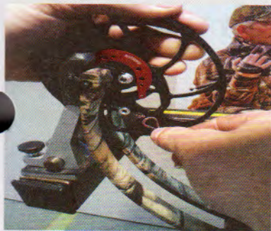
Step #19 Attach the 2nd buss cable to top cam post.
