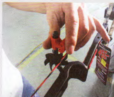
Step #20 Hook buss cable into cable slide or roller guard.
