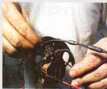
Step #19 Attach the 2nd buss cable to top cam post.
